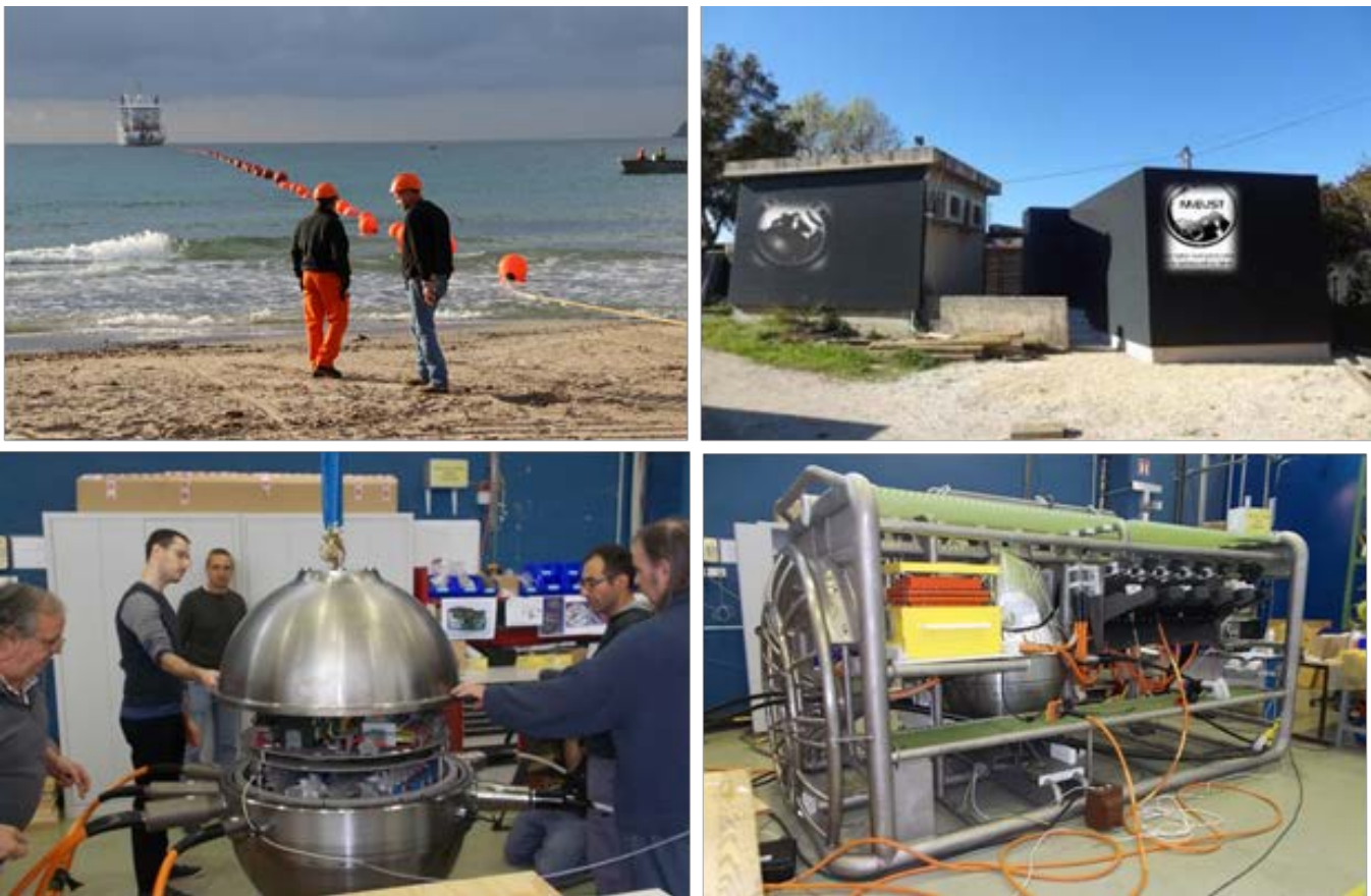
Fig. 5. The main components of the MEUST infrastructure: the shore power hut (top right); the MEOC under deployment in December 2014 (top left); the first node under final assembly in the CPPM hall (bottom right) with a zoom on the closure or the Junction Box (bottom left).
