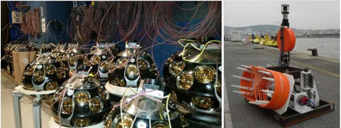
Fig. 1. Examples of scientific instruments to be connected to MEUST. Left: the 18 DOMs of the first neutrino KM3NeT DU in calibration in the CPPM dark room before integration as a DU; right: the EMSO ESS MII module integrated at the CNRS-INSU Technical Division.
